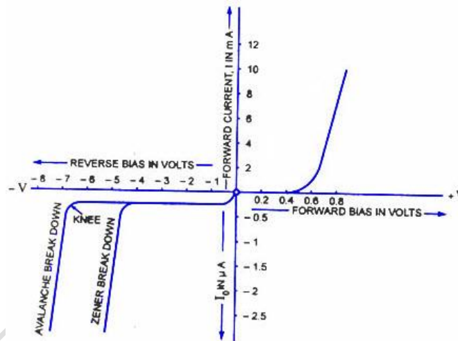
Figure :zener diode Characteristics
